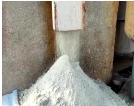
SOLID WASTE FROM PUSHER CENTRIFUGE
